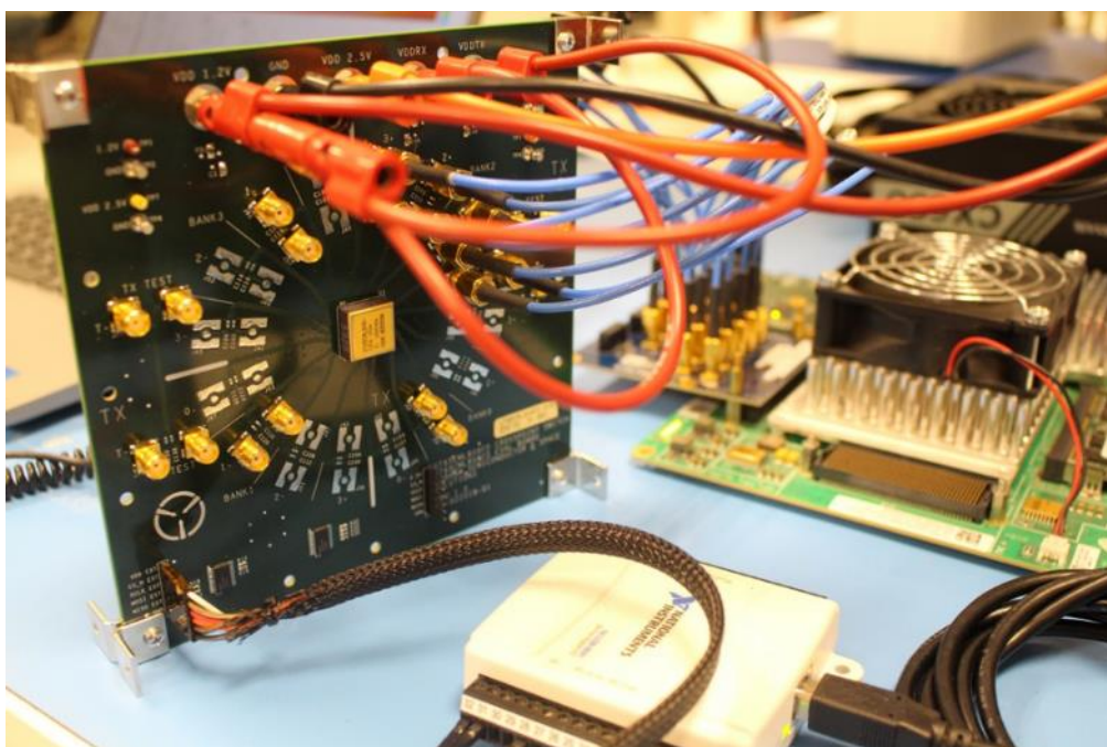
Figure 2: Test Setup – XPS+XQRKU060 Loop-Back Test: XPS EVB
