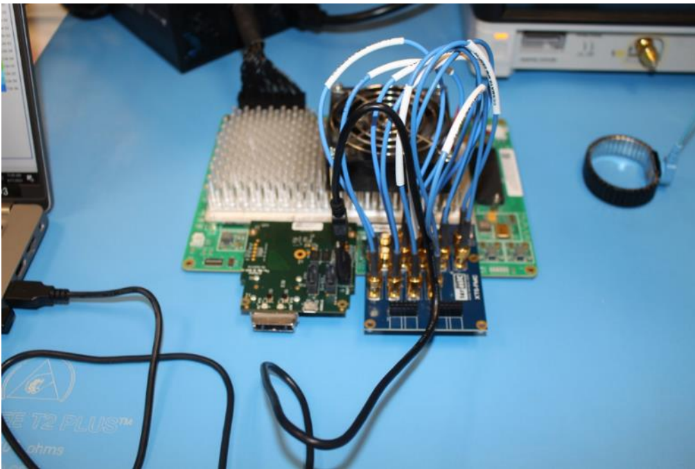
Figure 6: Test Setup – XQRKU060 SERDES Only Loop-Back Test Bench
